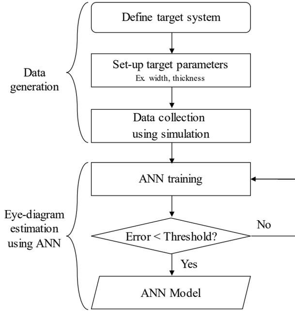
Fig. 2. Flowchart of data generation and training for the proposed ANN-based eye-diagram estimation method .
