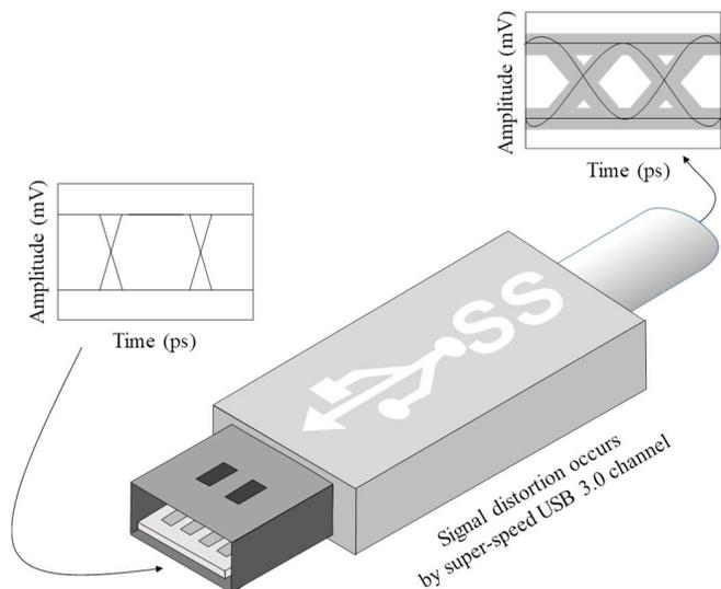
Fig. 1. Signal distortion occurred by USB 3.0 channel. The distorted signals can cause the system to malfunction.
