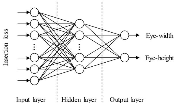
Fig. 3. The proposed ANN model for estimating eye-width and eye-height.
