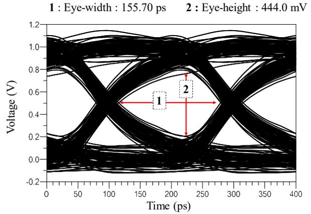
Fig. 6. Transient simulation results for verification of the proposed method.
