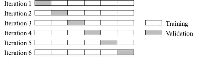
Fig. 4. K-fold cross-validation method applied in the proposed method.
