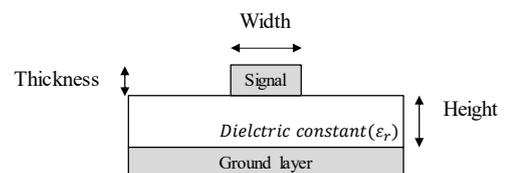
Fig. 2. Target channel and target parameters for Bayesian optimization
