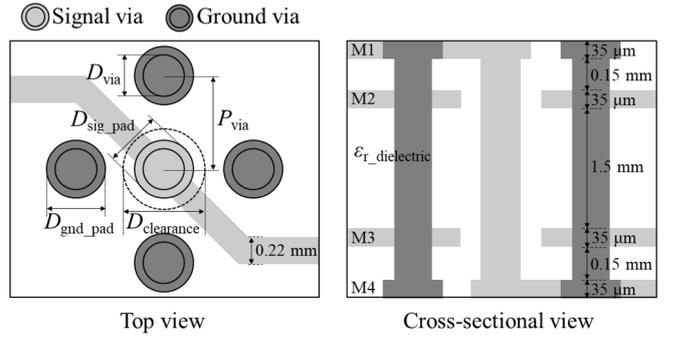
Fig. 3. Geometry and design parameters of THV in 4-layer PCB.
